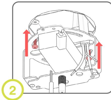
Screw bracket onto junction box.
