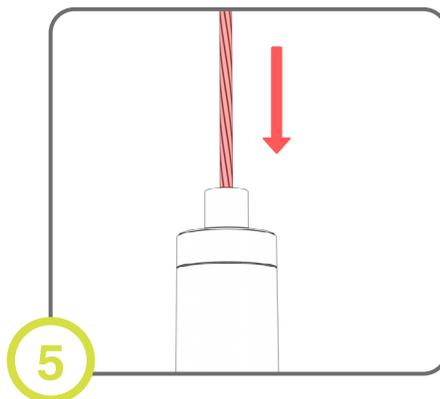
Adjust height by pulling aircraft cable through gripper on fixture. Cut excess cable.
