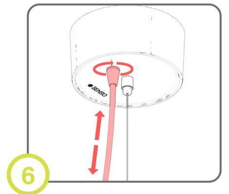
On canopy, adjust length of feed cable and tighten with cord gripper.
