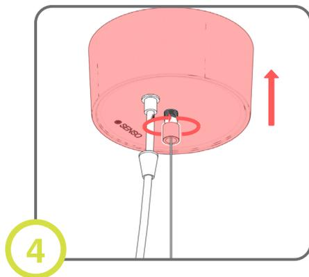
Slide canopy onto bracket and tighten aircraft coupler.
