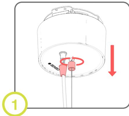
Unscrew grip cap and couplers, and separate canopy from bracket.
