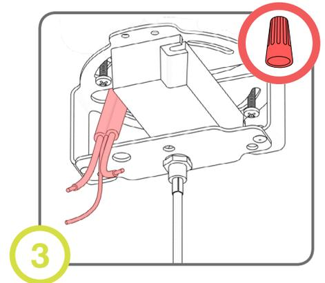
Pull cable from junction box and make electrical connections (refer to wiring page)
