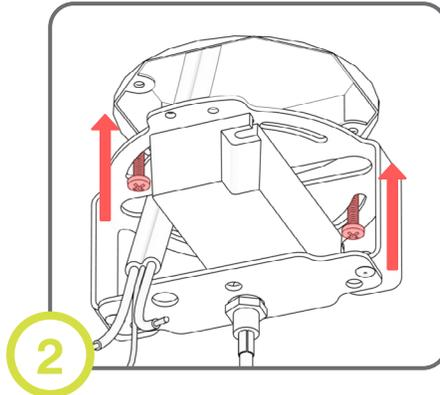
Screw bracket onto junction box.
