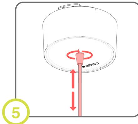
Adjust length of feed cable and tighten with cord gripper.
