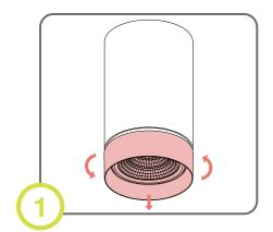
Hold the shade. Then hold baffle and rotate counterclockwise to remove it.
