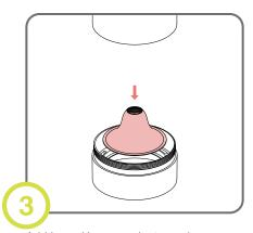
Add Lens, Honeycomb etc, and new reflector to baffle.
