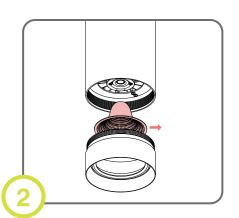
After seperate baffle from shade, remove reflector.
