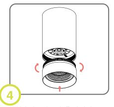
Hold shade and turn baffle clockwise to finish install.
