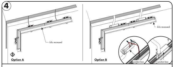
Option A: Run the fixture(s) lead wire to the remote power supply. Refer to page 3 for wiring.
