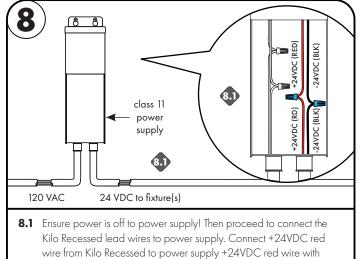
appropriate wire nut. Connect -24VDC black wire from Kilo Recessed
